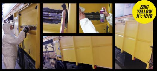
Bristol Waste approached U-POL about a problem with rust on their fleet of 284 collection vehicles, caused by acidic waste materials corroding the metal.
