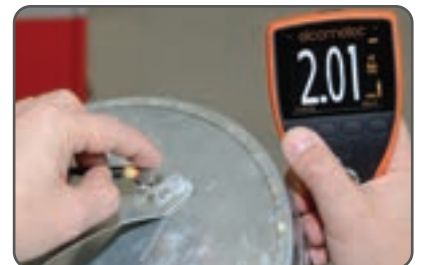
A maximum of 100,000 readings can be stored in the meter's memory
