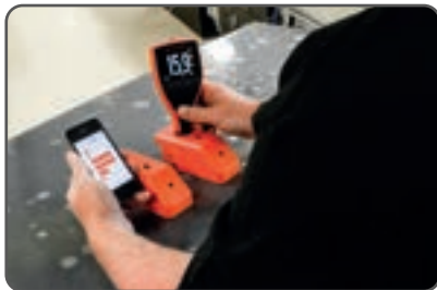
Ideal for measuring dry film thickness on thin coated substrates
