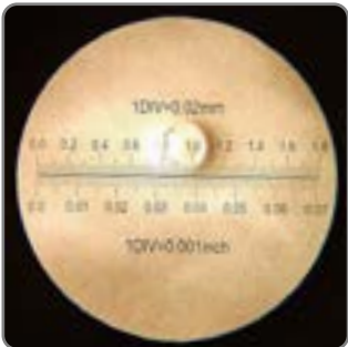
300 micron paint crater appearance
