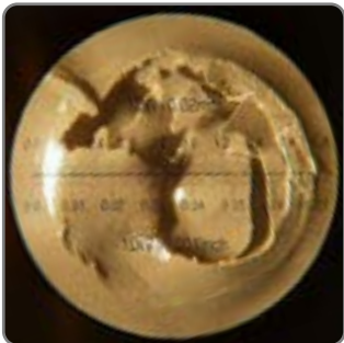
Appearance of air bubbles in primer coat
