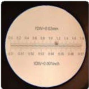
Appearance of speck of impurity in compressed air of 80 microns
